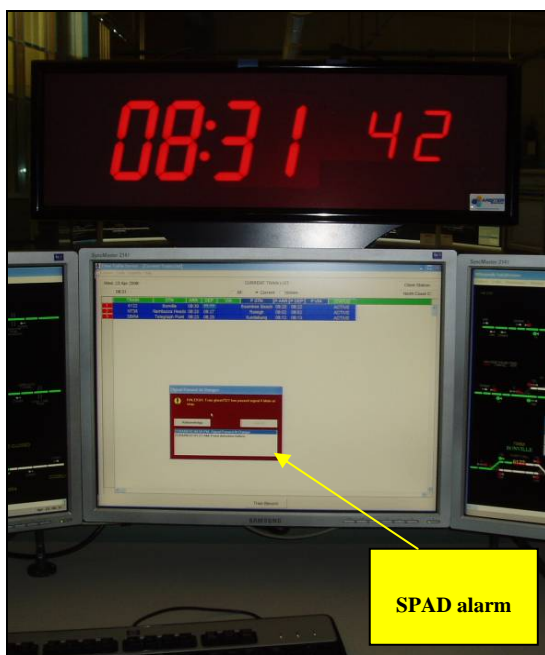
Figure 3: Example of visual SPAD alarm at Broadmeadow Train Control Centre
