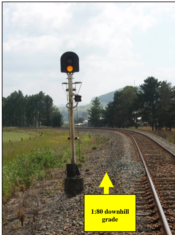
Figure 4: Down distant signal at Gloucester
