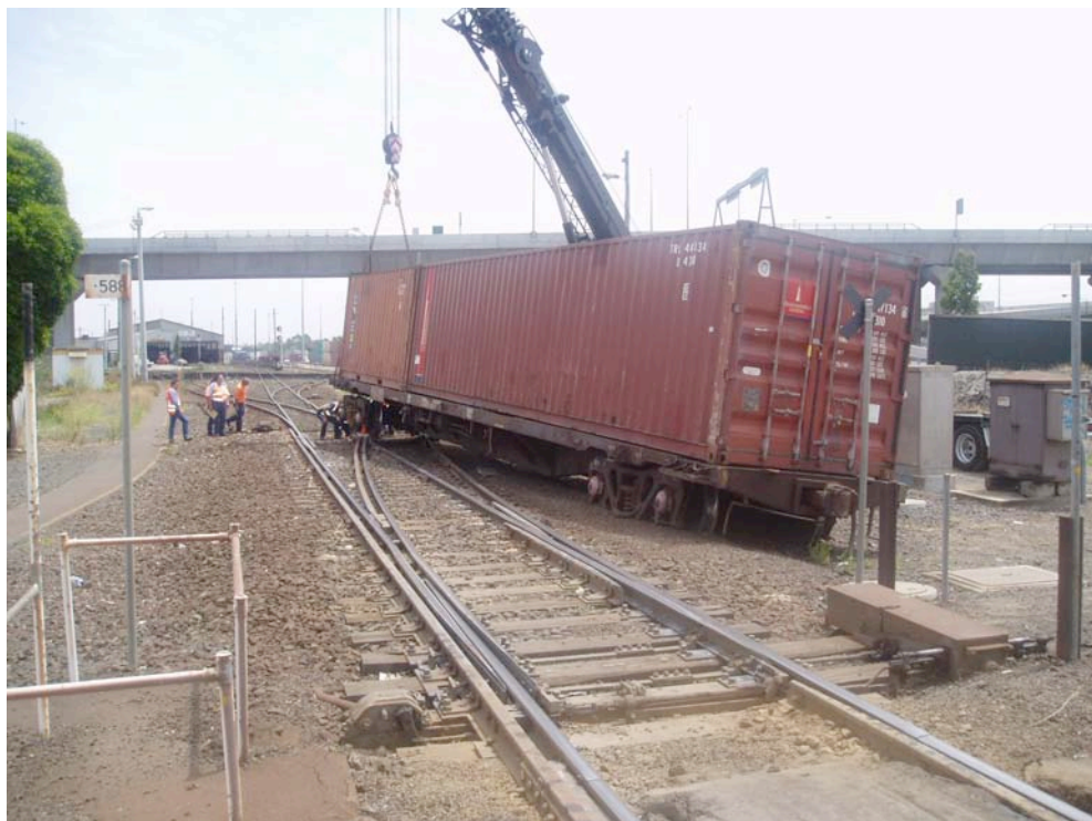
Figure 8: Recovery of rear-most wagon RQSY 34384B, in its final stopping position, being carried out following the removal of the XPT on Thursday 20 January 2005.
