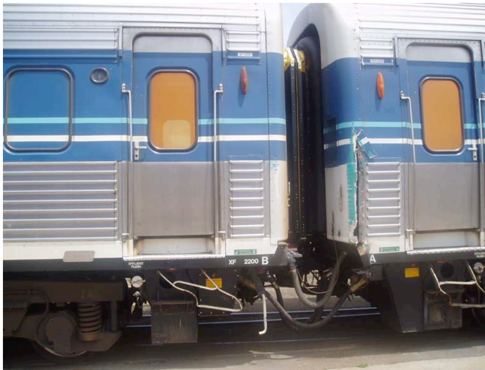
Figure 7: Example of fibreglass and door step damage to XPT cars C and B.
