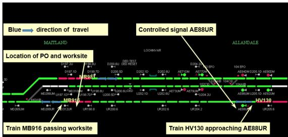
Figure 2: Extract of Phoenix replay showing indications displayed to the network controller at 1022 on 30 October 2015.
