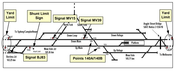
Almost immediately, the network controller realised that he had simultaneously authorised passenger train SN57 into the Up Platform Road and train D231 into the Up Refuge Siding. This meant that both trains were to traverse a common set of points (140) which would bring the two trains into direct conflict.
