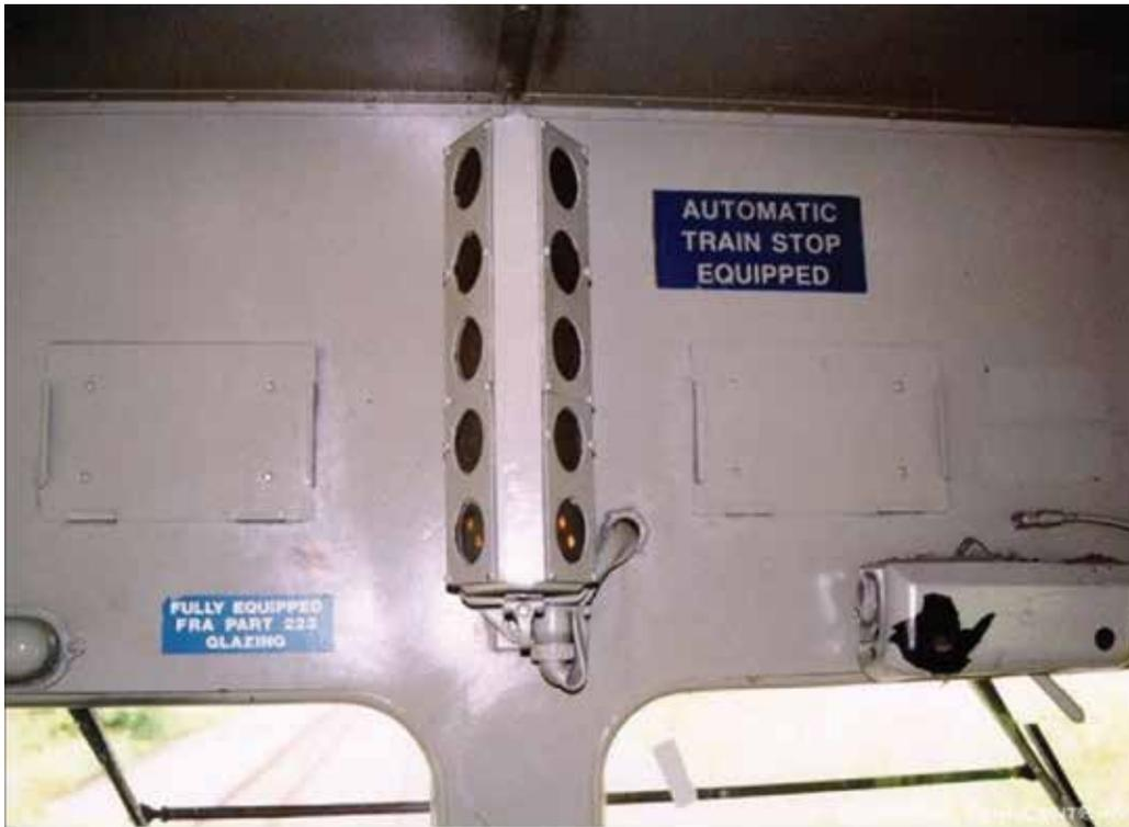
**Photo 2.** Typical locomotive cab signal display (Source: Railway Technical Web pages, [www.railway-technical.com](http://www.railway-technical.com))
