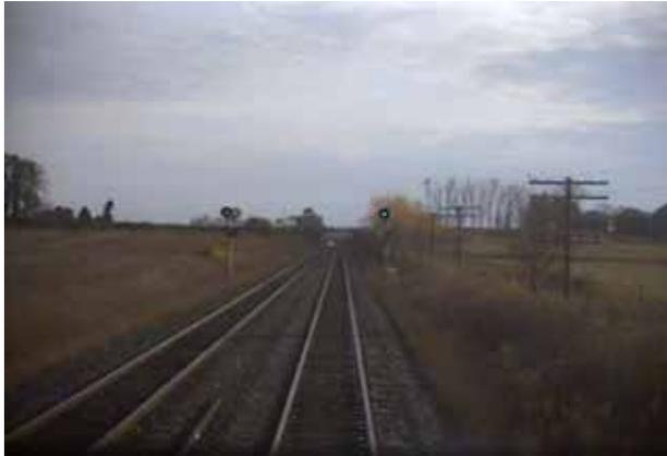
Photo 4. Still frame of locomotive forward-facing video at 10:13:22 (Note: Top light appears to be yellow.)
