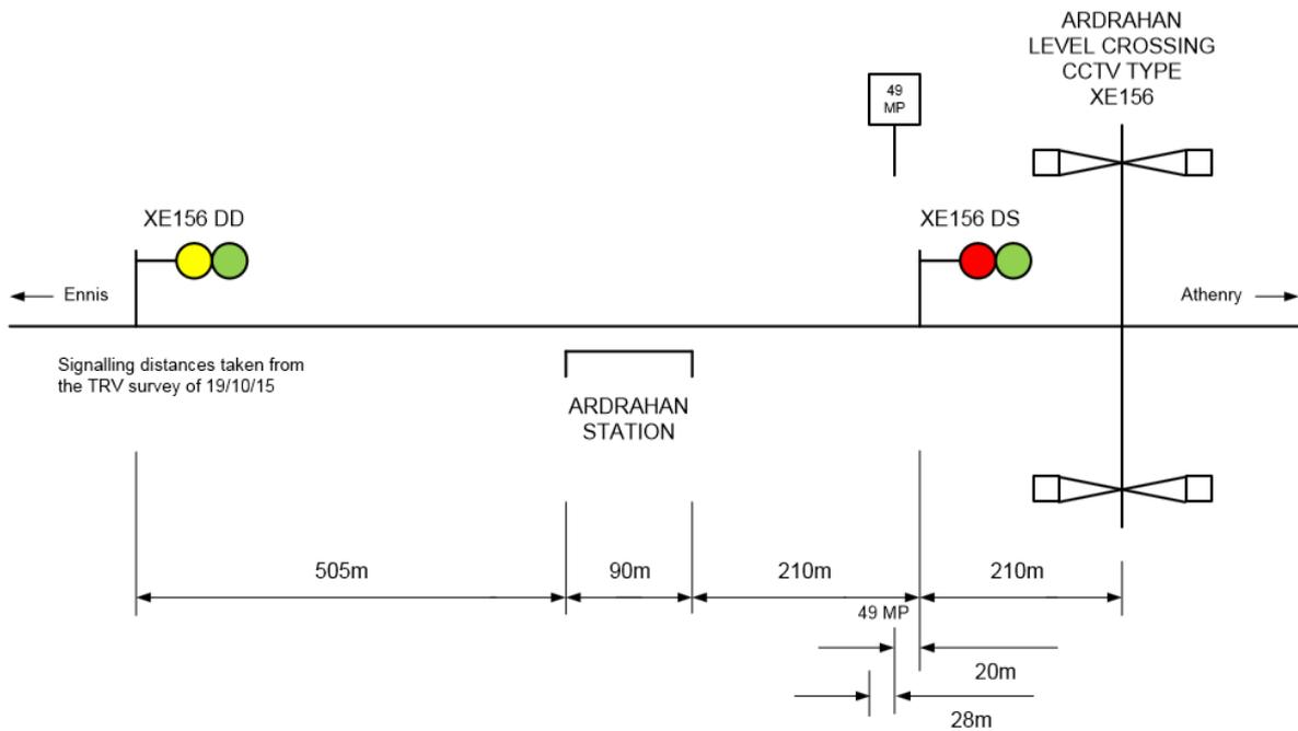
Figure 6 – Signal layout at Ardrahan
