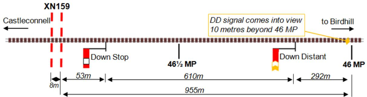
Figure 21 – Layout of signals at XN159
