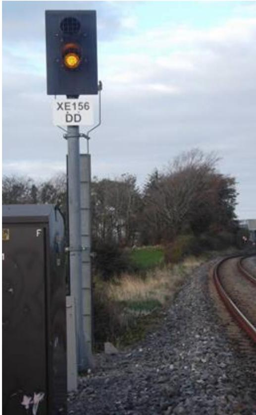
Figure 4 – Distant Signal XE156DD
