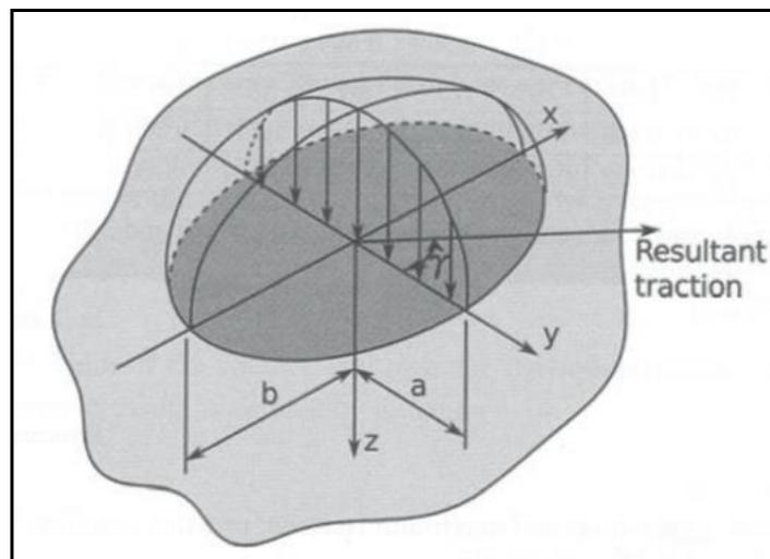
**Figure 29 – Elliptical contact patch – circa 1 – 1.5 cm<sup>2</sup>**
