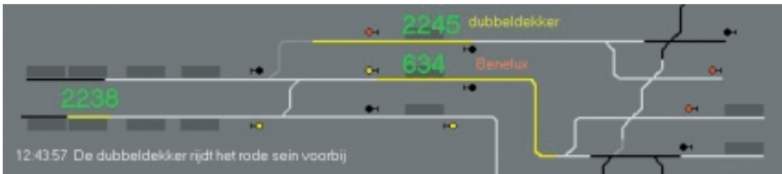
Figure 3. All changes in the system: the occupation of sections, changes of signals, etc. are all automatically recorded. On this basis, it is possible to precisely determine what happened in Dordrecht. The figures indicate the train numbers. The grey rectangles have no relevance in this figure. The light-grey lines indicate the sections of set routings. The yellow lines indicate the sections occupied by a train. At the indicated moment, the double-decker passed the signal at red. The section after the signal issued a track occupied message. The Benelux train is at that moment still in front of the signal, on the routing set for it. This course of events is visible on the train controller's monitor. Train number 2238 is the train approaching on the adjacent track.
