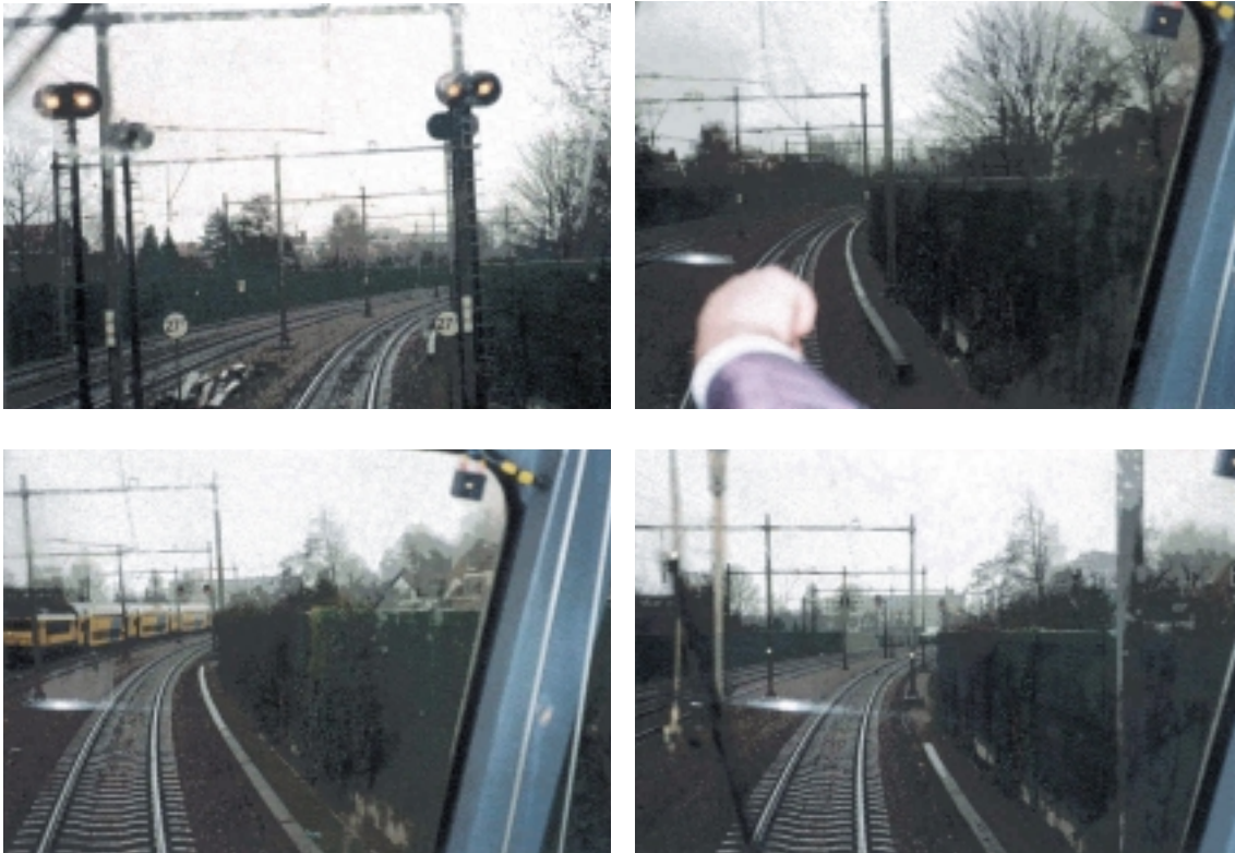
Figure 10. The view of signal 1132 at 200, 178, 140 and 120 metres before the signal, determined two months following the collision. In this period, the trees have few leaves. This is not the case throughout the year. During the passage by the double-decker on 28 November, the central signal for the Benelux train was at green.
