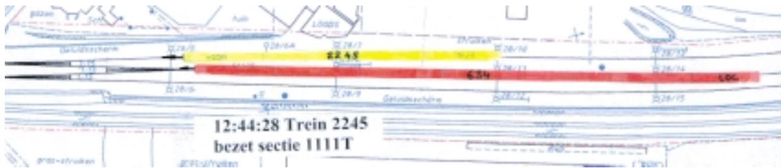
Figure 5. The Benelux train is still behind the double-decker, 21 seconds after the double-decker has passed signal 1132.
