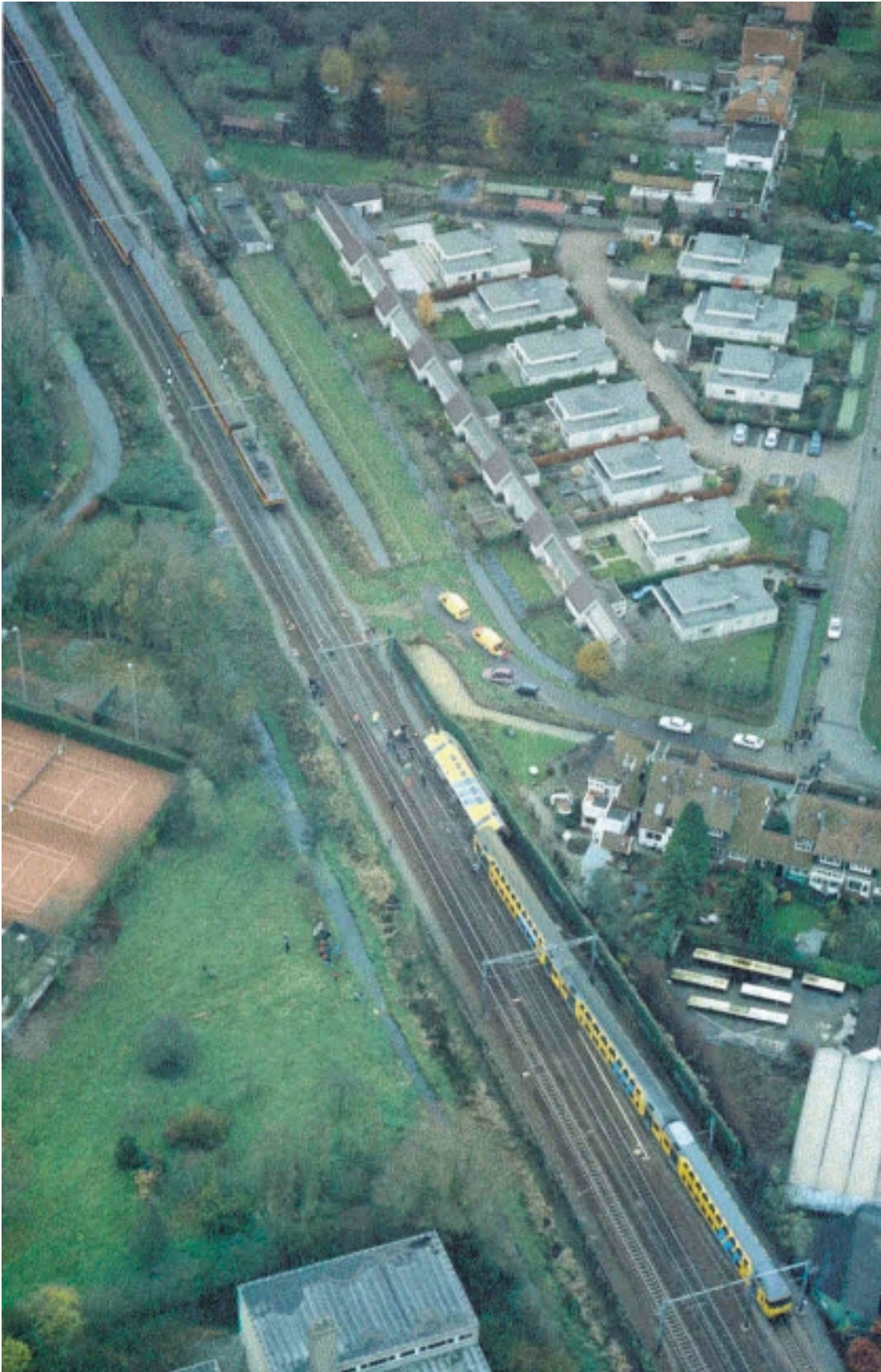
Figure 7. Overview of train positions following the collision. In the top left-hand corner, we see how the carriages of the Benelux train are blocking the adjacent track. A potentially very hazardous situation.
