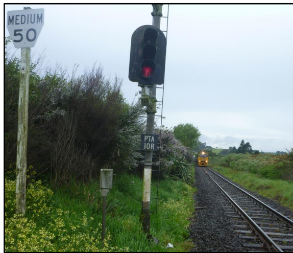
Figure 3 Signal 10R at 'Stop'
