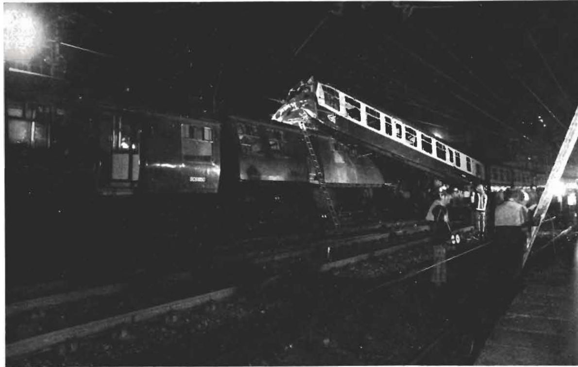
Photograph No. 1. General view of site of collision showing leading coach of DMU on top of leading coach of EMU.
