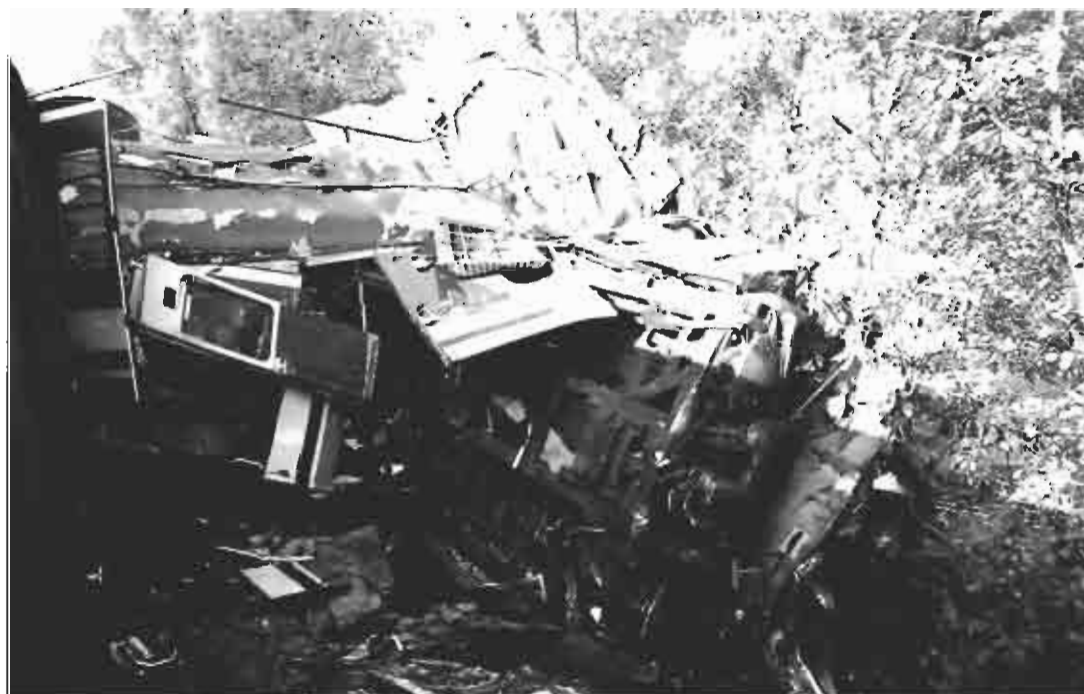
The overturned leading coach of the Down train with the wreckage of the leading coach of the Up train lying above it
