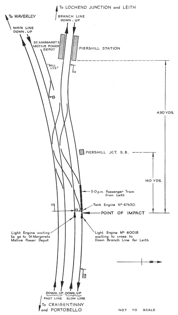
The mistakes which the signalman made were that he failed to send the "Blocking back inside Home signal" to Lochend Junction, and that he omitted to put collars on his Up Main to Slow, and Up Branch to Slow Home signal levers. Thus, when he forgot the light engine, there was nothing to prevent a train being offered from Lochend Junction, or to prevent him accepting and pulling off the signals for it.
