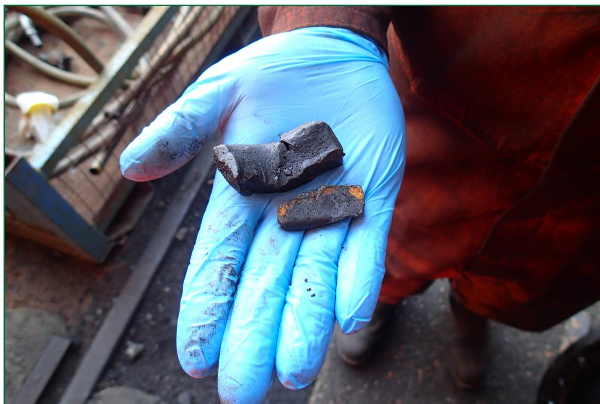
Figure 10: Remains of cotter from piston rod
