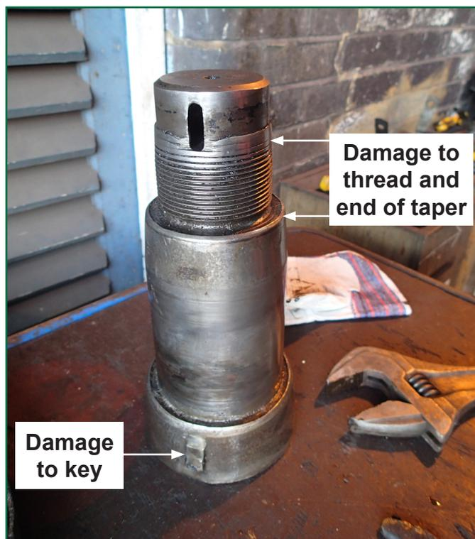
Figure 8: Gudgeon pin of 'Tangmere' after the accident
