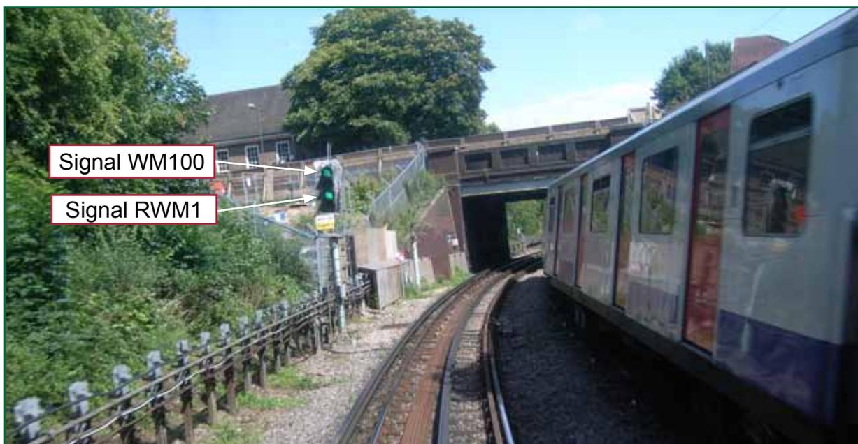
Figure 5: Signal WM100 mounted above signal RWM1. Signal WM1 is beyond the road bridge ahead
