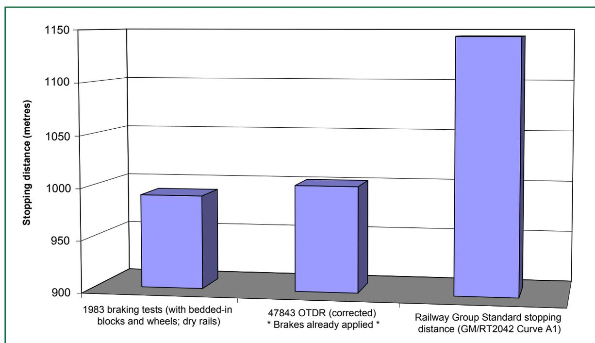
Figure 9: Comparison of stopping distances from 75 mph (121 km/h)
