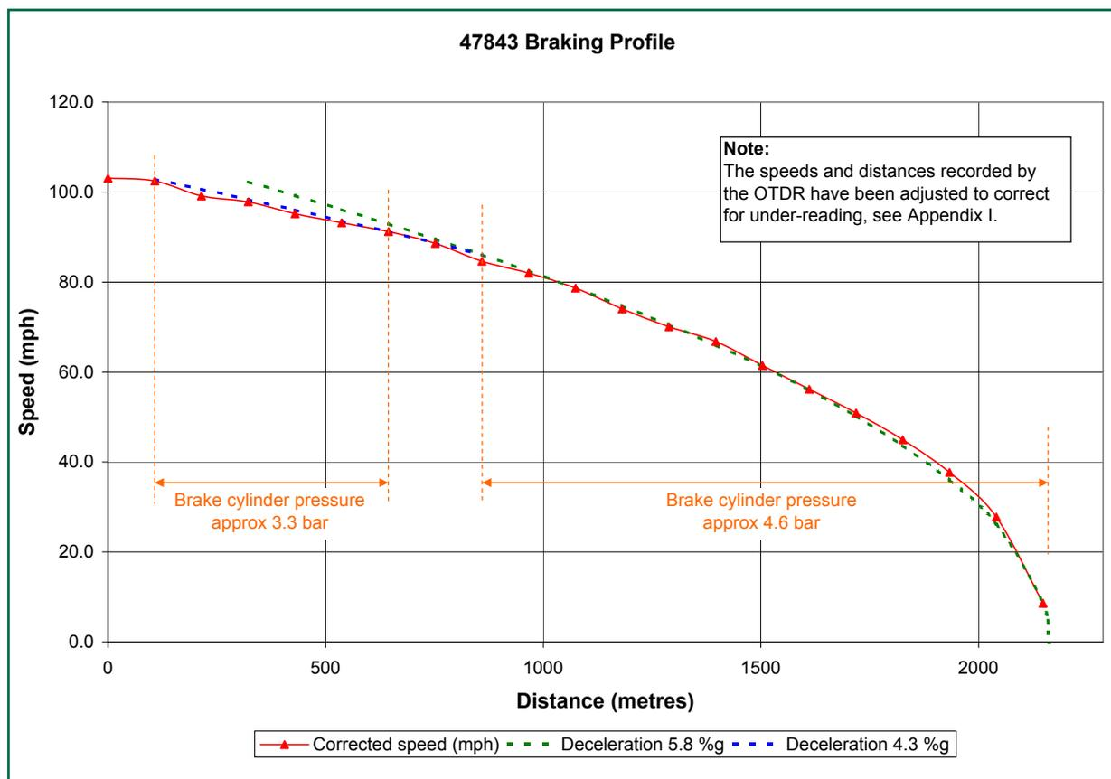
Figure 7: 47843 braking profile
