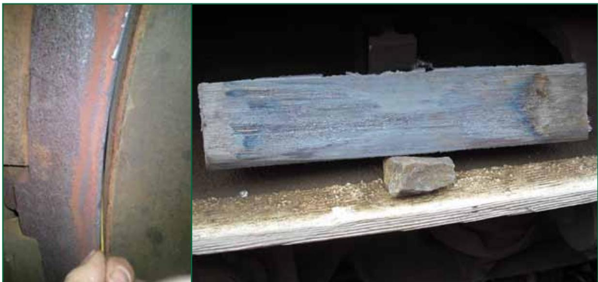
Figure H1a and H1b: Brake blocks from locomotive 47843, when examined after the incident (courtesy URS and RTL)
