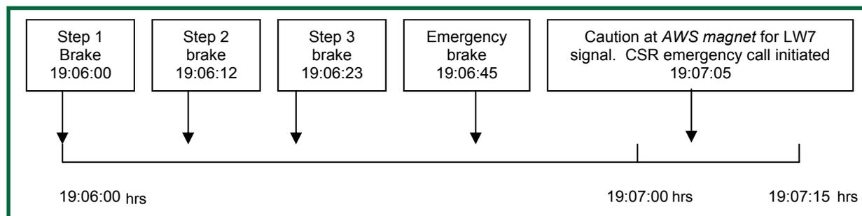
Figure 3: Timeline of key events before driver of 2D45 made CSR emergency call to signaller.
