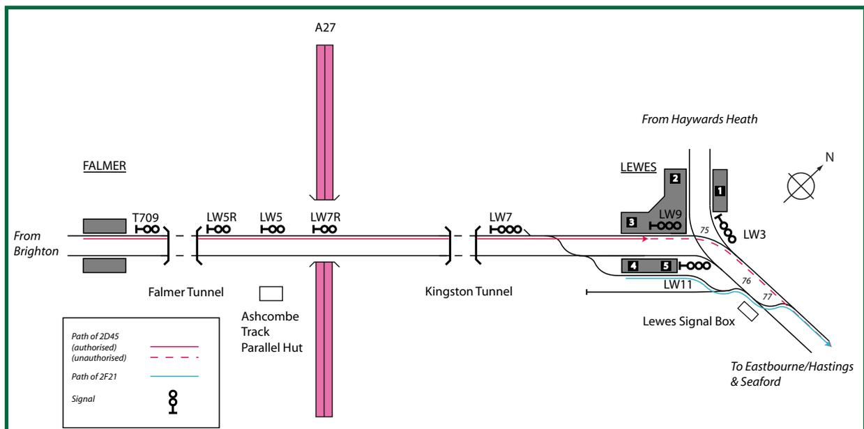
Figure 2: Track layout showing location of incident.
