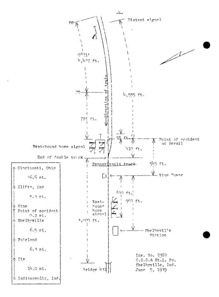
The distant signal is electrically operated. A time release is provided so that when this signal is cleared and placed again in the normal or caution position, the derails or switches within the limits of the interlocking cannot be changed until three minutes have elapsed.
