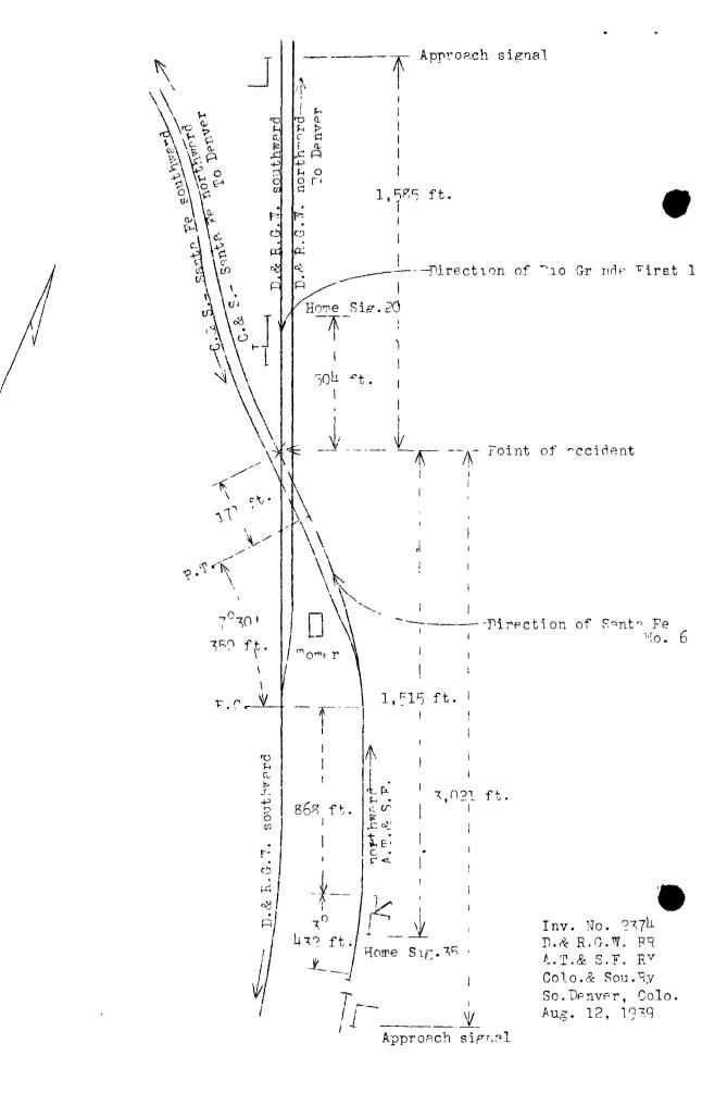
length, a tangent 868 feet in length, a 7030' curve to the left 350 feet in length, and a tangent 171 feet to the crossing. The grade for north-bound trains is 0.31 percent descending a distance of 1,300 feet then level 1,950 feet, 0.9 percent descending a distance of 250 feet, and then level a distance of 100 feet to the crossing.
