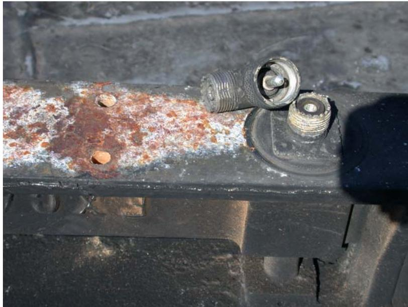
**Figure 2.** Corroded cable connection on locomotive UP 1966.
