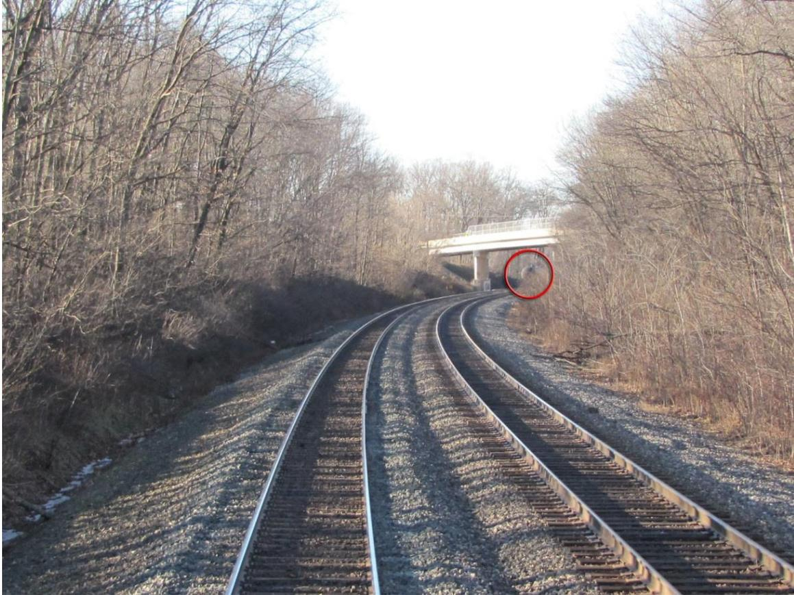
**Figure 6.** Rear of exemplar standing train (circled) is first visible at about 1,304 feet away.
