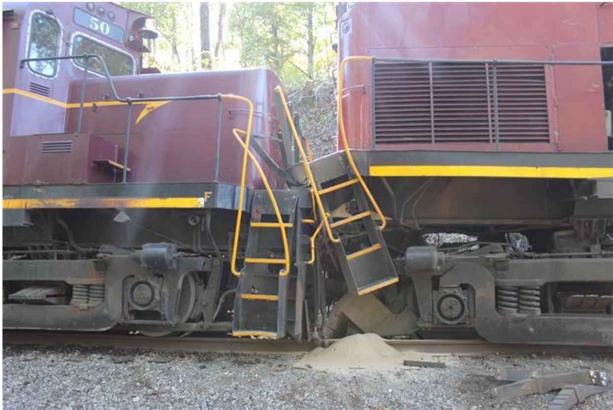
Figure 2. Locomotives of work train (left) and excursion train (right) after collision.
