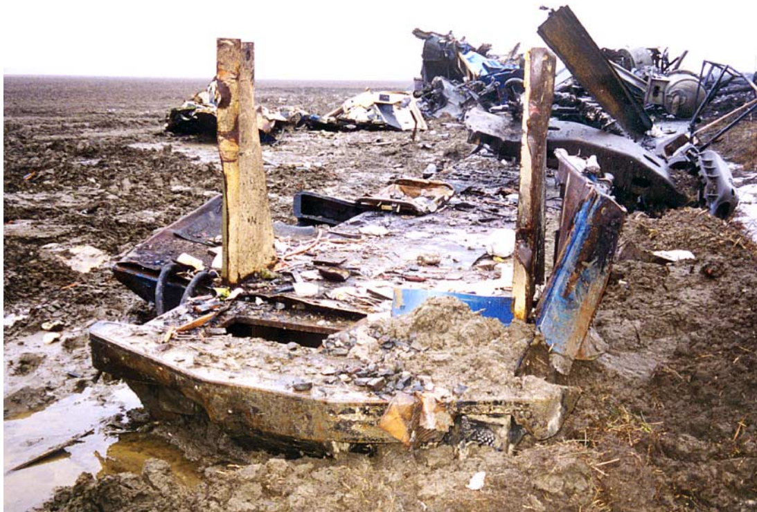
Figure 6. Locomotive underframe assembly.
