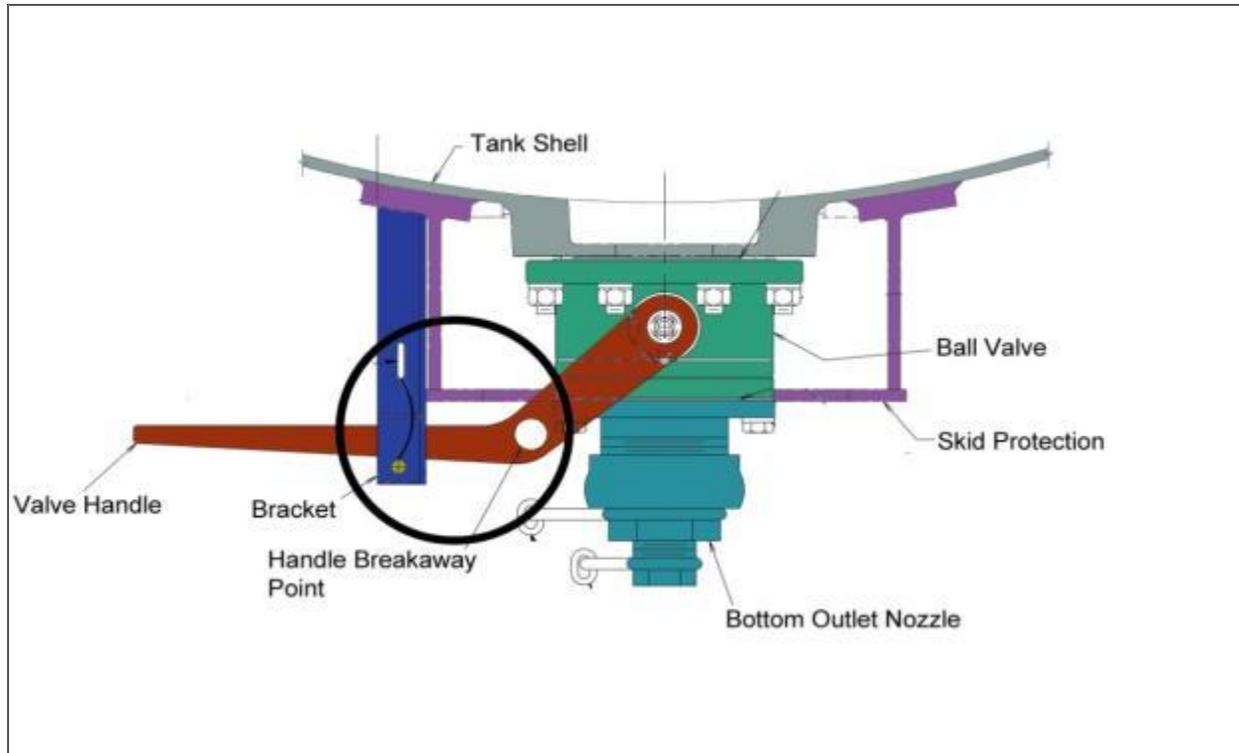
**Figure 7.** Bottom outlet valve configuration, as modified from original design, for derailed CITX and CTCX cars. (Not to scale) The operating handle securing bracket is circled. (Adapted from a Trinity Tank Car drawing)
