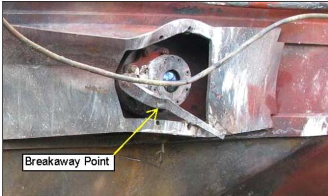
**Figure 11.** Bottom outlet valve of car CTCX 731599 showing exposed valve and bent but intact valve operating handle. Handle retaining bracket is missing. (Valve was opened during derailment but was closed by emergency responders.)
