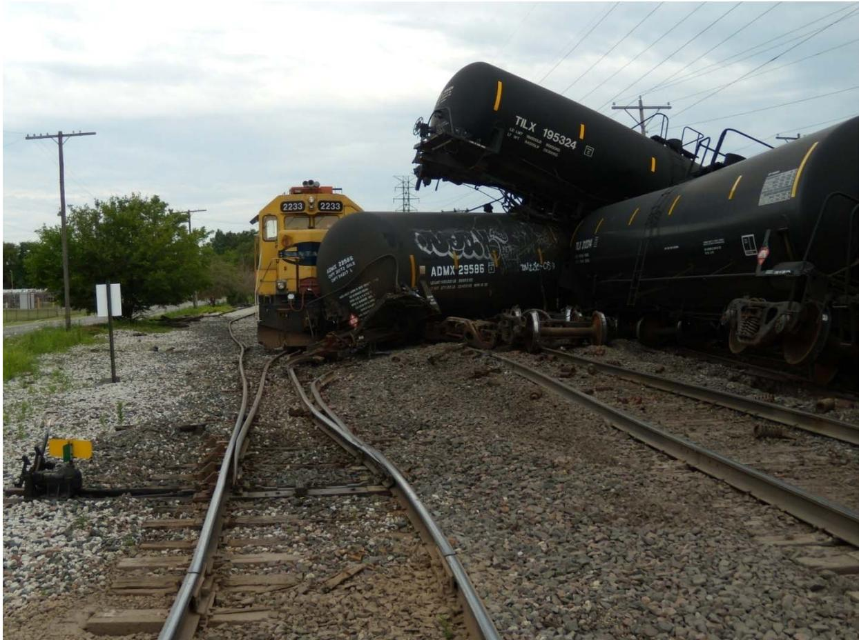
**Figure 6.** Wreckage of DME tank railcars.
