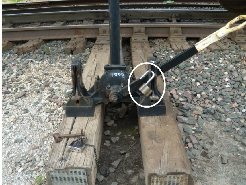
**Figure 7.** Bettendorf Yard north yard hand-operated switch with unlocked BNSF lock.
