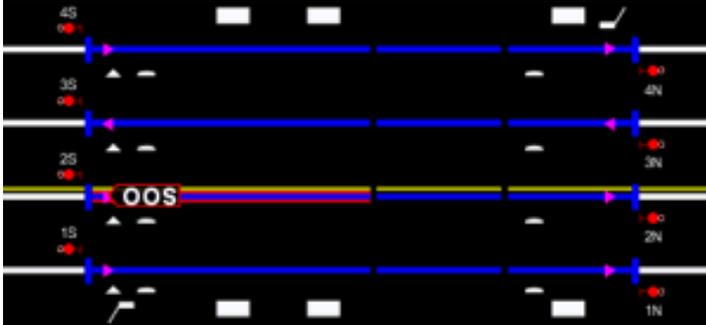
**Figure 4.** Dispatcher's display screen at 7:25 a.m. showing tracks 1–4 between Control Points Baldwin and Hook. Track 2 is out of service track (magenta), and tracks 1, 3, and 4 have electronic blocks (blue).
