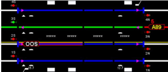
**Figure 7.** Dispatcher's display screen at 7:47 a.m. with train 89 on track 3 shown by the A89 designation.
