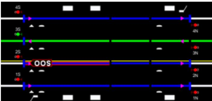
**Figure 6.** Dispatcher's display screen at 7:34 a.m. with a clear signal for train movement on track 3 indicated by the green highlight.
