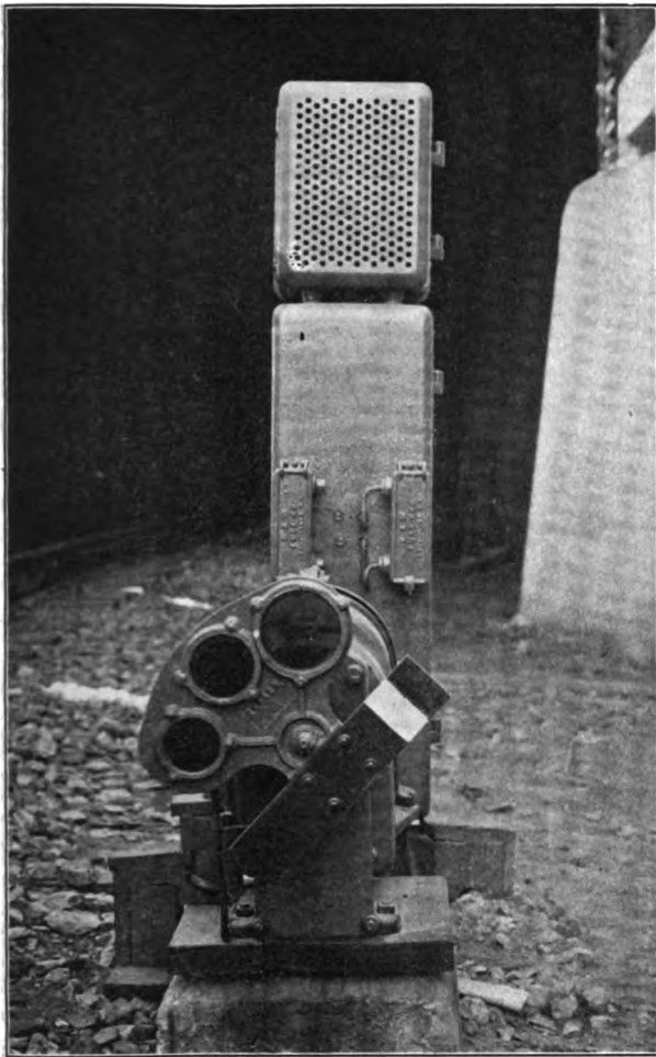
Fig. 7—Three-Position Dwarf Signal.
