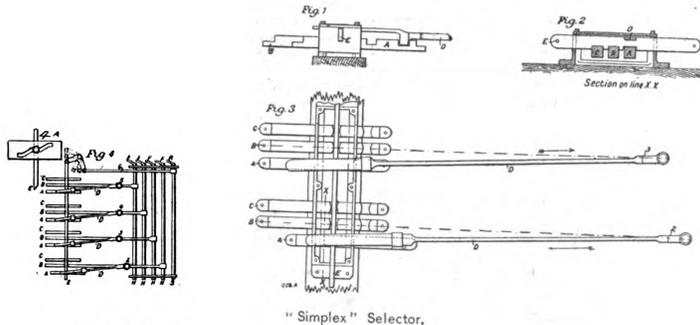
Used in Interlocking Machine at Waterloo Station—London & Southwestern Railway.
