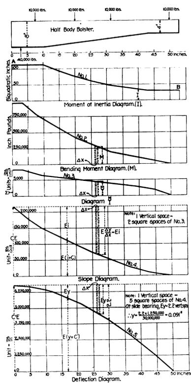
Fig. 3.—Diagrams for Deflection of a Body Bolster.
