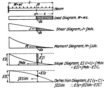
Fig. 2.—Graphical Methods for Bolster Computations.
