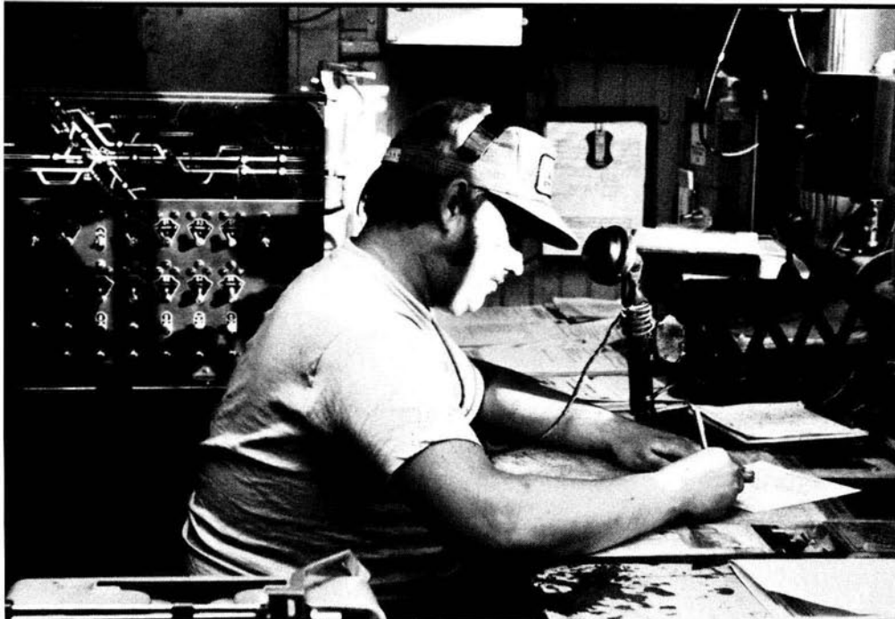
OPERATOR at West Liberty, Ia., "copied three west" (above) for 57's train, the Extra 351 West, which picked them up at speed from the order stand (right). To ease dispatchers' load, Rock had several local-control CTC installations like this.
