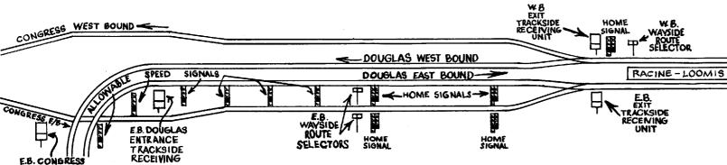
At Loomis Junction, Douglas trains diverge from the median strip west-bound and converge with the median strip eastbound. Two separate interlocking plants, one for each direction of traffic, are provided to permit the various train movements at this location. These interlocking plants operate independently of each other, so that a failure in one direction of traffic will not affect train movements in the other direction of traffic.
