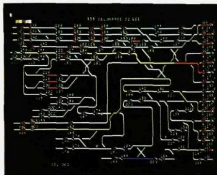
Fig. 8 A set train route is marked with a green line on the display screen and a shunting route is marked with yellow or blue alternatively
