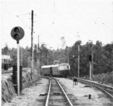
Fig. 5 X 4162 Exit northwards from Stockholm E left, entrance signal H to first block section; middle, between tracks, rear view of dwarf signal; further to the right, entrance signal A^{1\frac{1}{2}}
