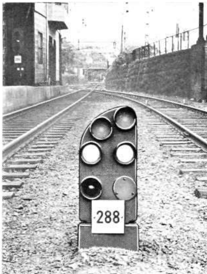
Fig. 3 Position-light shunt signal with four white apertures and one green
