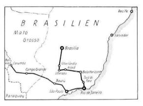
The carrier system is type ZAA 8 for eight telephone channels. Over a distance of nearly 500 miles the circuit runs on the only open-wire pair that exists between Campo Grande and Baurú. This line belongs to the railway and was built for telegraphy; it is an entirely untransposed 3.2 mm copper wire line with the wires spaced about 16 inches apart and follows the railway through the most desolate country.
