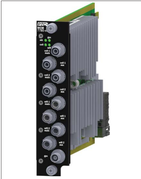
Picture 1 Onboard Wireless Communications Module, containing dual LTE modems, dual Wi-Fi modems, a GPS receiver, and Gigabit Ethernet backplane connectivity.
