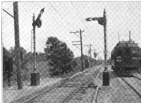
Fig. 8. Semaphore Signals—"Proceed" and "Stop."
