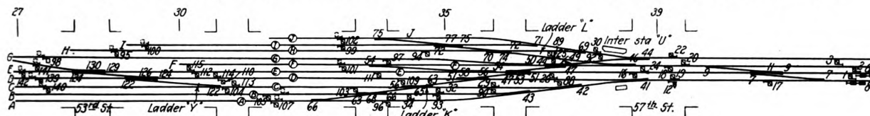
The Track Plan of Tower "U," Showing the Switch and Signal Locations
