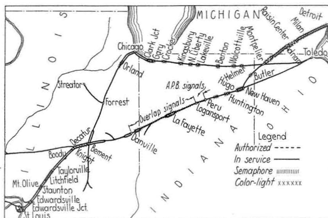
Wabash main line between St. Louis, Chicago and Detroit showing principal automatic block and station signaling
