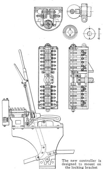
the controller is effected by a compensating ball and cam that takes care of any variable action in the locking shaft.
