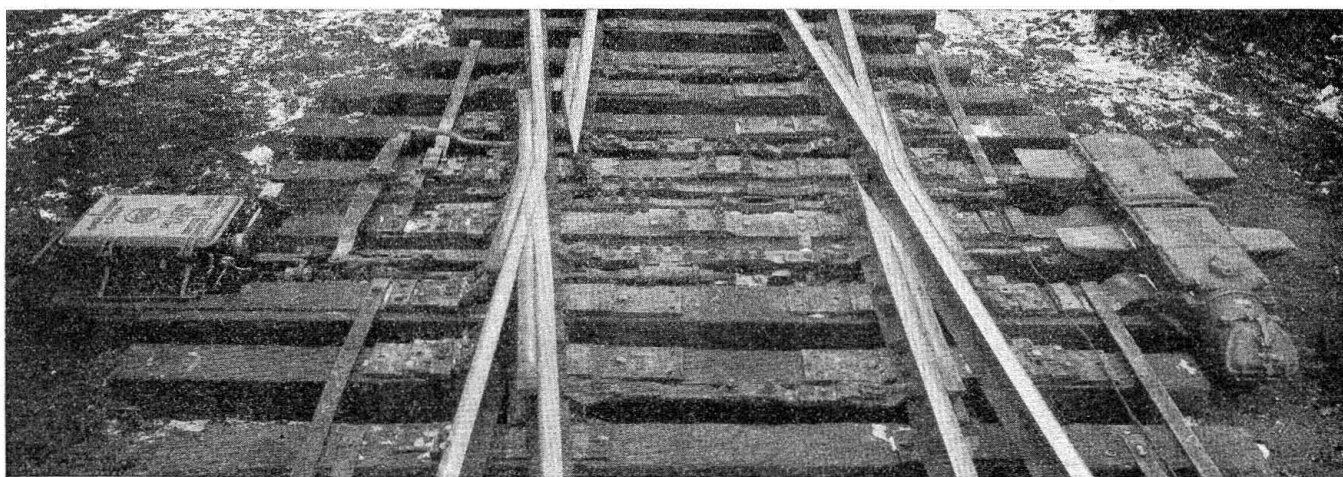
Crossing frogs with movable points are operated by a Model-5A switch machine equipped with a dual-selector mechanism
