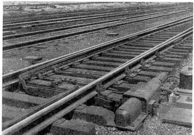
Electro-pneumatic switch movement with CP valve
