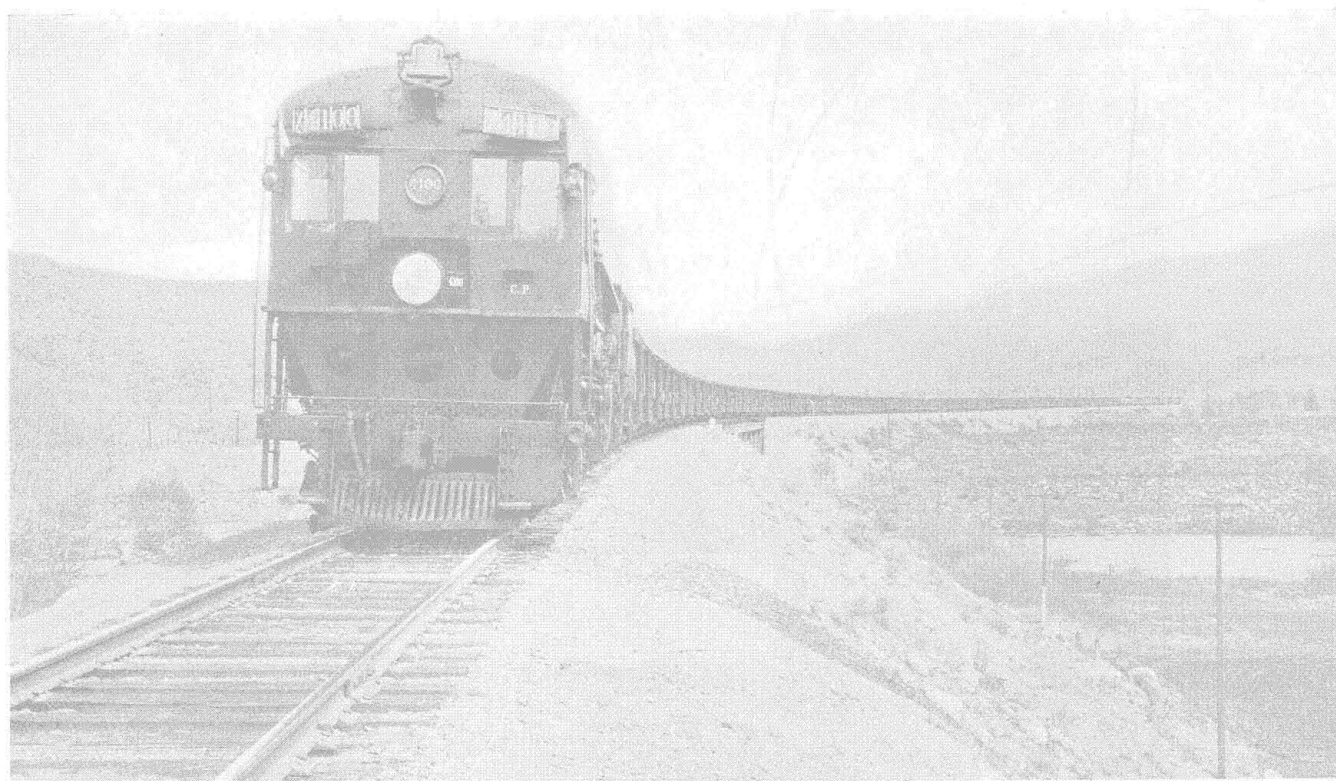
Southern Pacific train in the Sierra Nevada mountains, hauled by one of the New 4-8-8-2 type single-expansion articulated locomotives built by Baldwin
