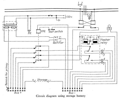
transformer taps. An outstanding advantage of this scheme is that a completely charged storage battery stand-by is available regardless of the number of train movements.
