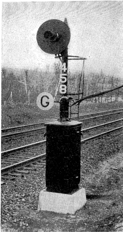
Typical three-aspect automatic block signal with grade marker
