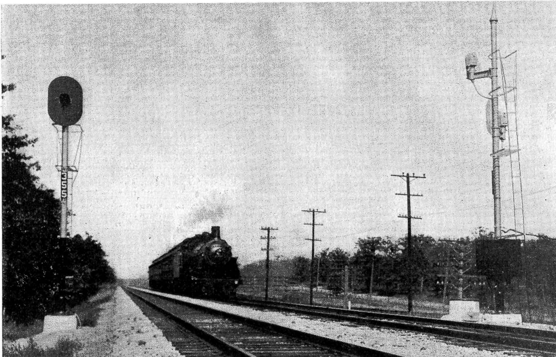
The North Western operates left-handed and the signals are located at the left of the running track—Three-aspect searchlight signal at left and four-aspect searchlight signal at right
