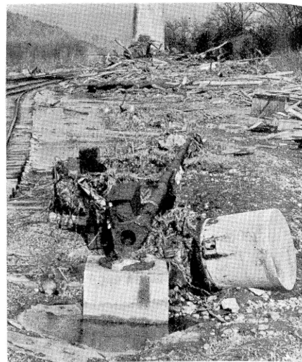
The base casting of this B. & O. semaphore was broken
