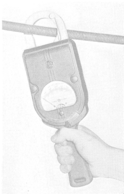
Type AK-1 hook-on volt-ammeter in use for current reading
