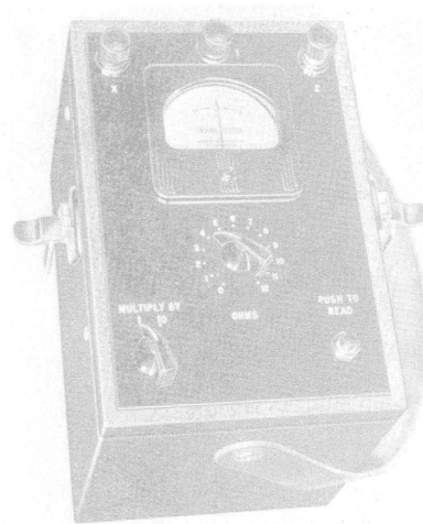
Model 251 vibroground with the lid removed
