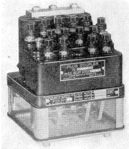
Top view—relay minus coupler, center-view—coupler, bottom—plug coupler applied to DN-11 relay
