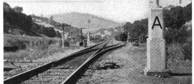
Above — High dwarf and hand-throw derail on a turn-out where the mainline switch is operated by switch stand
